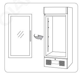
6. Disassemble the right upper hinge.
