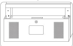
3. Cut the slot on the front panel and install the hinge inside.
