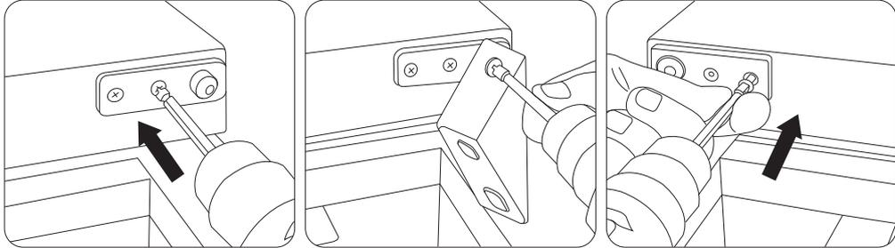
6. Remove the castor support board, right front castor, and left front castor consecutively. Then install back the right castor. (Tool: socket spanner)
