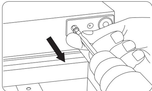
5. Reverse the door. Install the previously removed spring hinge on the left top and auxiliary hinge on the left bottom.
