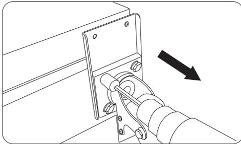
7. For the hinge axis on the castor support board, remove it from the right and install on the left .
