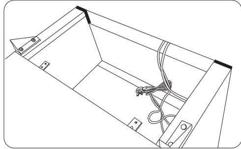
2. Remove the right upper hinge and left upper hinge. (Tool: socket spanner)
