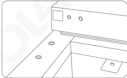
4. Remove the door from the right lower hinge . Now remove the auxiliary hinge.
