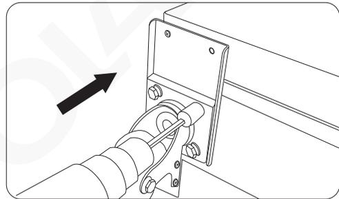
9. Install the previously removed left top hinge on the right top. (Tool: socket spanner)
