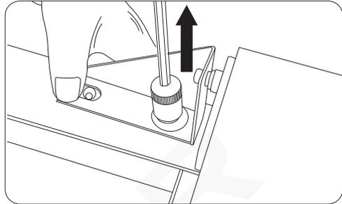
3. Remove the spring hinge on the right top.
